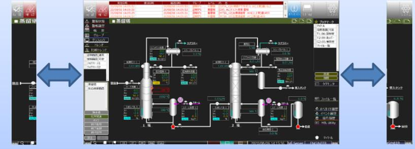
Uses a variety of screen modes to make information easier to see. You can perform operations tailored to the user in 1-screen mode, 4-screen mode, and screen pop-up. **It also has a number of other functions.**
